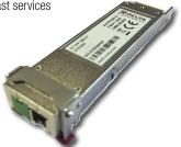
The OT XFP 1550 09 transmitter modules can complement or replace today's legacy 1310 nm and 1550 nm broadcast transmitters.
